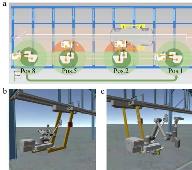
Fig. 4. (a) Bottom view of vehicle mounting - swivel module extended; (b) VR-view - retracted swivel module with screwing robot in home position; (c) VR-view - extended swivel module with screwing robot in working position.
