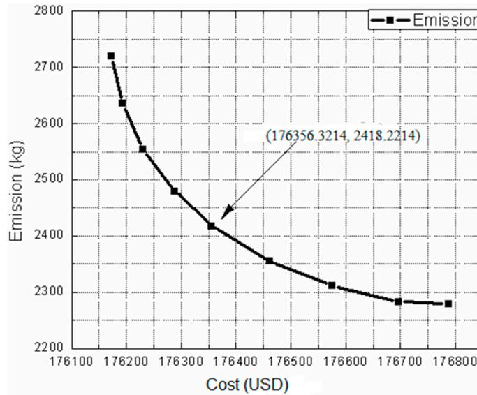
Fig. 1. Cost vs. Emission using HMGWO (without RES).
