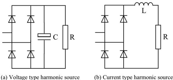
Fig. 25. Two types of harmonic source nonlinear loads.
