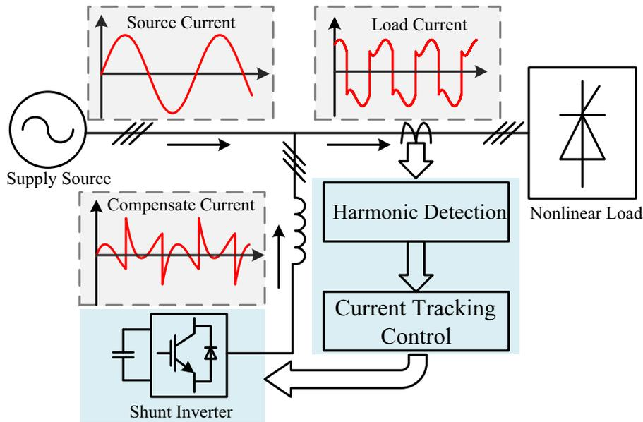
Fig. 2. The principle block diagram of APF.
