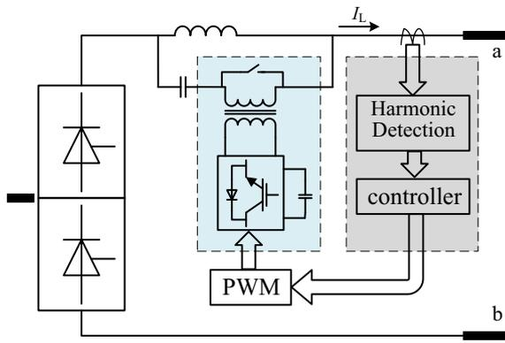
Fig. 24. the active DC filter series equipment of HVDC system.
