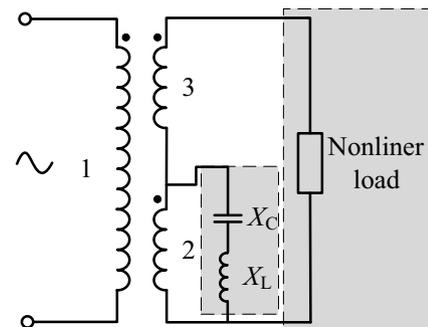
**Fig. 20.** Harmonic suppression single-phase traction transformer.
