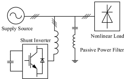
Fig. 15. The combination configuration of shunt APF and shunt PPF.
