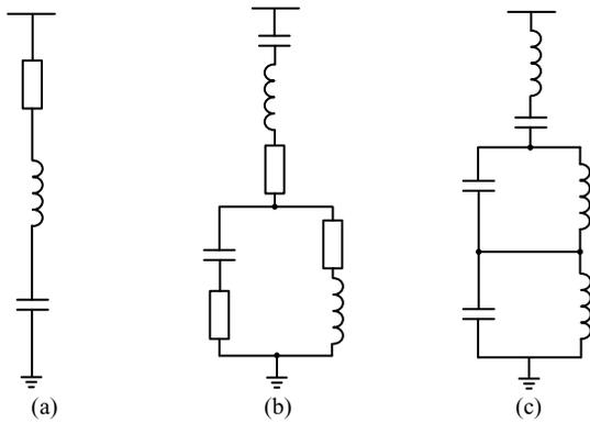
Fig. 3. Common PPFs. (a) Single-tuned filter. (b) double-tuned filter. (c) triple-tuned filter.
