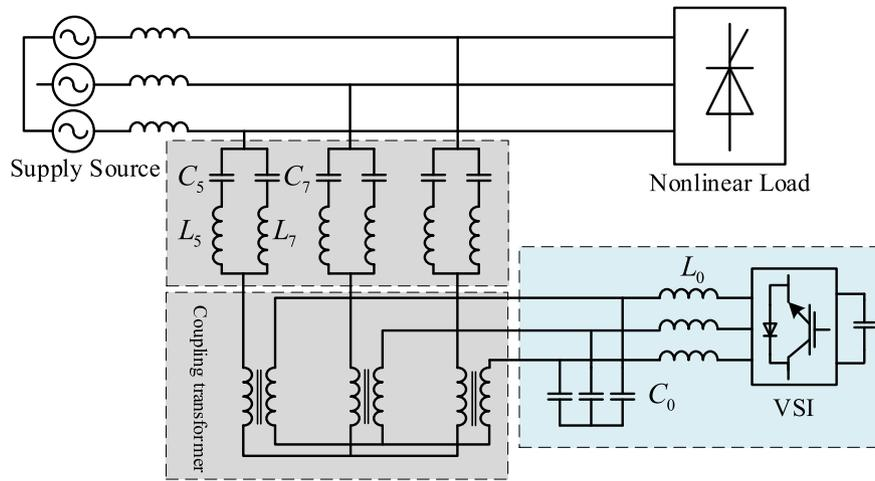
Fig. 14. The configuration of series APF connected in series with PPFs.
