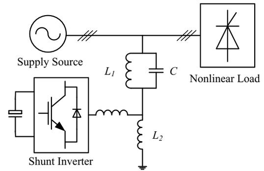
Fig. 7. The configuration of shunt APF with injection circuit based on shunt resonant of LC filter.
