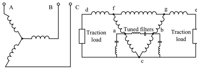
Fig. 21. Multifunction impedance matching and balance traction transformer.
