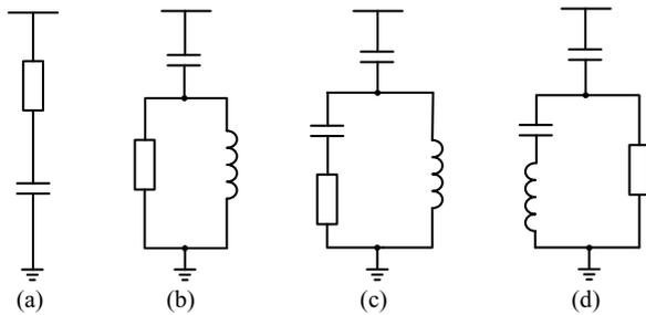
Fig. 4. High pass PPFs. (a) First order filter. (b) second order filters. (c) third order filters. (d) C-type damped filters.
