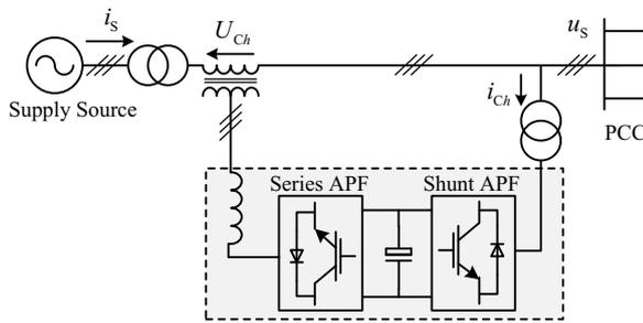
**Fig. 19.** The configuration of unified power quality conditioner.
