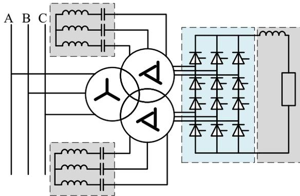
Fig. 22. Three phase multi-pulse rectifier and converter transformer.
