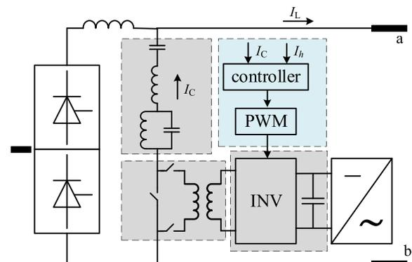
Fig. 23. The active DC filter parallel equipment of HVDC system.
