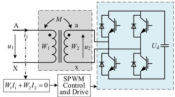
Fig. 17. The circuit of the series APF based on FMFC.
