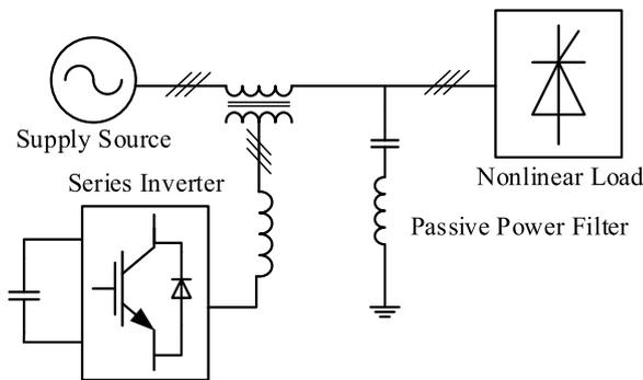
Fig. 16. The combination configuration of series APF and shunt PPF.
