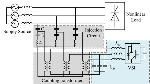
Fig. 8. The configuration of shunt APF with injection circuit based on series resonant of LC filter.
