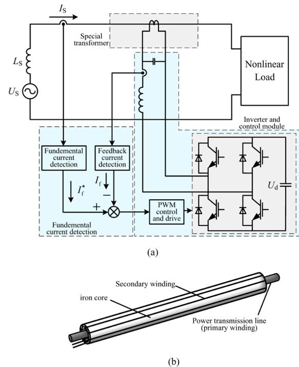
Fig. 27. The configuration of plug-and-play integrated modular series active harmonic isolator. (a) The circuit topology. (b) three-dimensional figure of special transformer.
