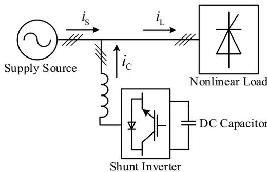
Fig. 5. The configuration of traditional shunt APF.
