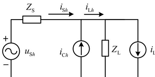
Fig. 6. The equivalent circuit of traditional shunt APF.
