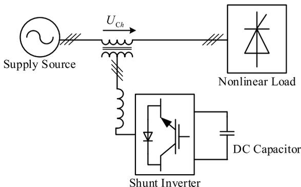
Fig. 12. The configuration of traditional series active power filters.
