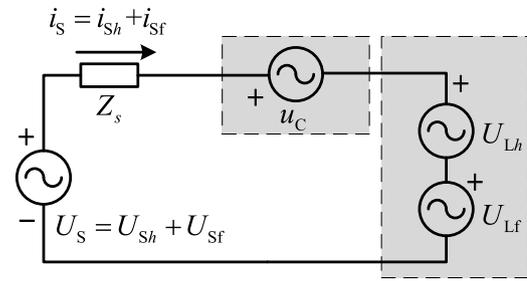
Fig. 13. System equivalent circuit (control approach of detecting source current).
