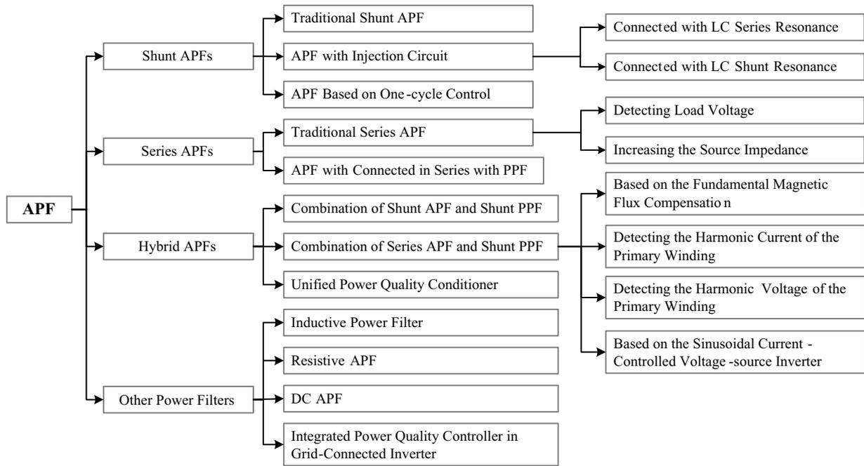
Fig. 1. Classification of active power filter according to power circuit configurations and connection.
