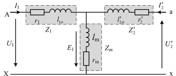
Fig. 18. The Equivalent-T circuit of series transformer.
