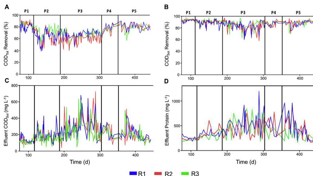
**Fig. 1.** Reactor process performance data for R1, R2 and R3, over the five phases, showing (a) the total COD removal; (b) the soluble COD removal; (c) the soluble COD concentration in the effluent; and (d) the protein concentration in the effluent.
