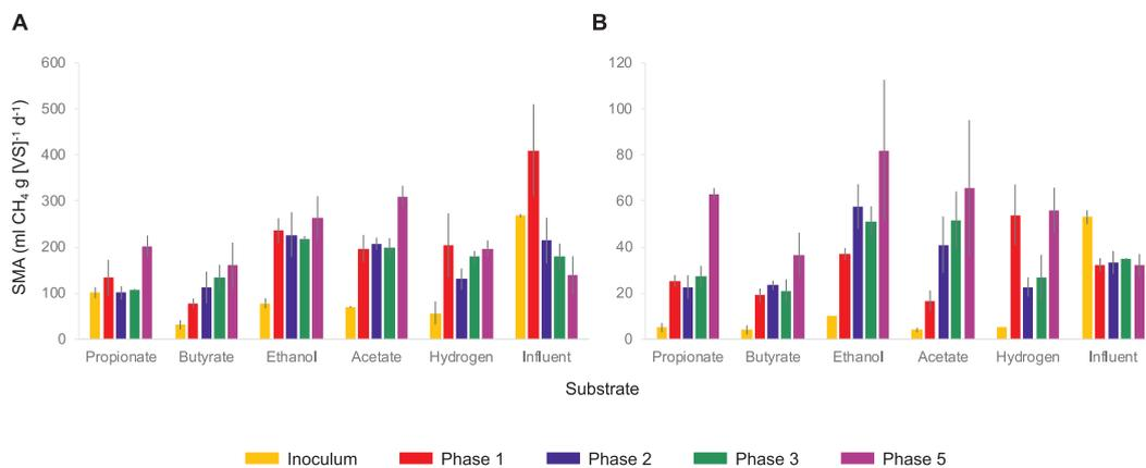
**Fig. 2.** Average SMA ( $n = 3$ ) of reactor biomass from the seed inoculum (day 0), and samples taken from P1, P2, P3, and P5, performed at (a) 37 °C and (b) 15 °C against methanogenic substrates: propionate, butyrate, acetate, hydrogen ( $H_2/CO_2$ ), and the reactor influent.
