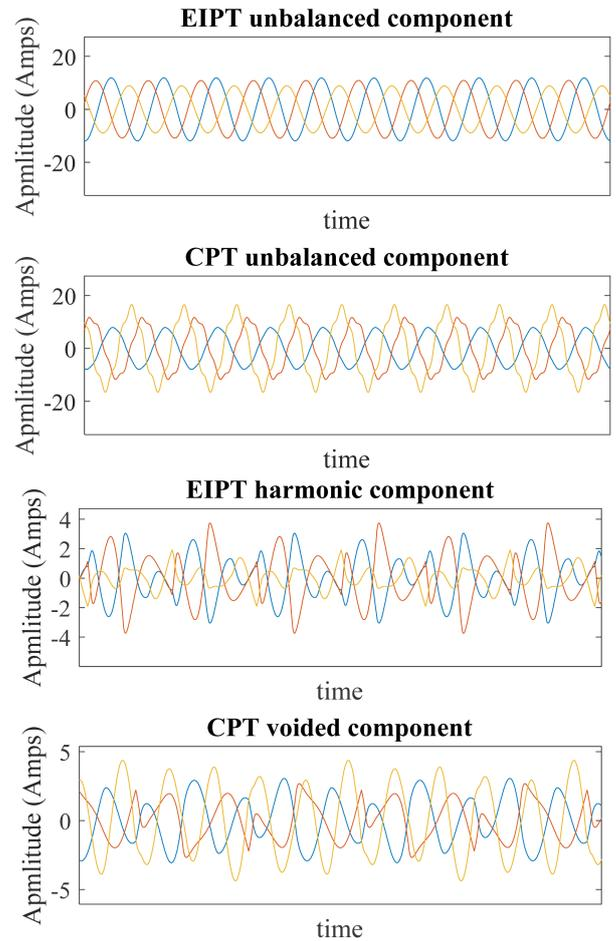
Fig. 10 Harmonic and unbalance current components in EIPT and CPT
