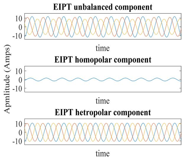
Fig. 11 Heteropolar and homopolar and total (heteropolar + homopolar) unbalance current components in EIPT
