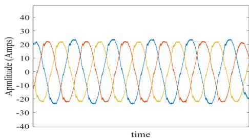
Fig. 15 Grid currents after compensation by using CPT
