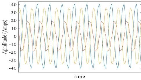
Fig. 8 Current waveforms of the load in phases a, b and c
