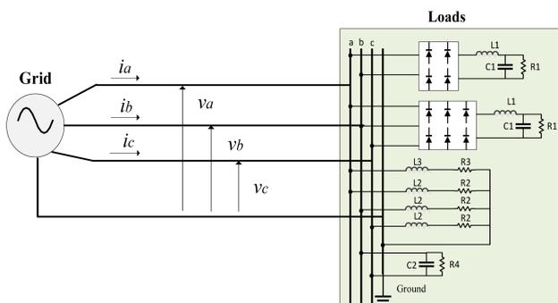
**Fig. 6** Three-phase four-wire system with different types of loads
