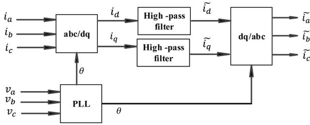
Fig. 4 Method for current decomposition
