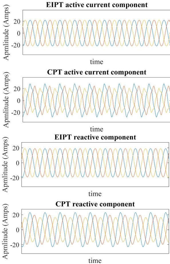
Fig. 9 Active and reactive current components in EIPT and CPT
