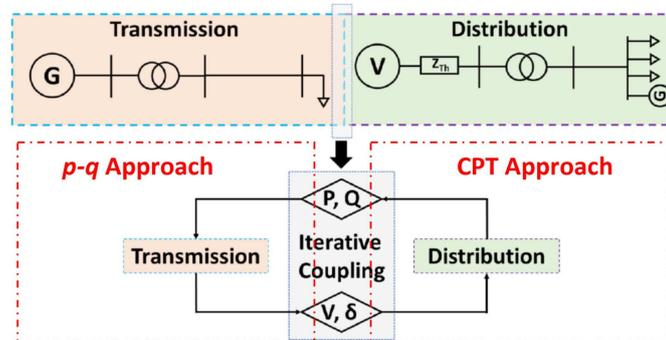
**Fig. 5**  $pq$  is the current trend of time-domain power theories in transmission level applications while CPT plays a major role in the distribution level and microgrid systems
