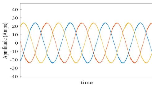
Fig. 14 Grid currents after compensation by using EIPT
