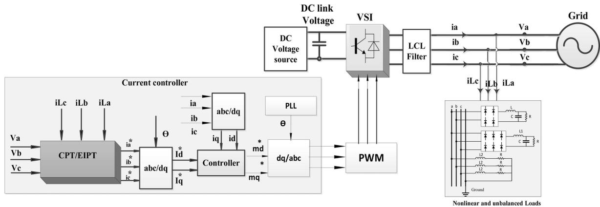
Fig. 12 Schematic diagram of the power conditioning system with CPT/EIPT
