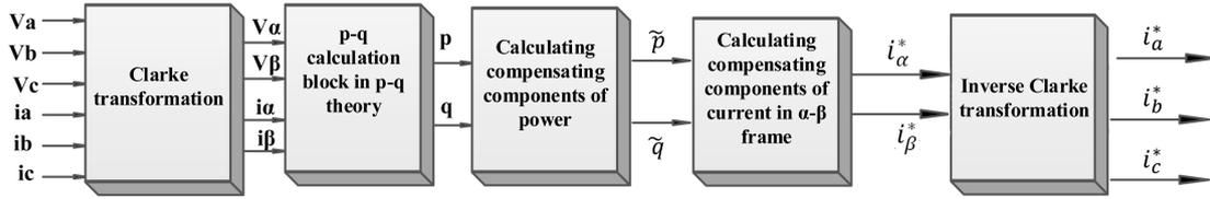
Fig. 3 Theory-based distortion compensation schematic
