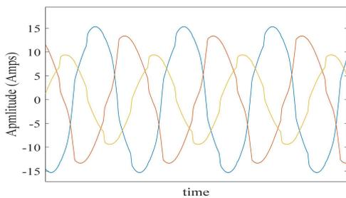
Fig. 13 Grid currents without compensation
