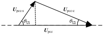
FIGURE 4. Harmonic voltage contribution evaluation diagram.
