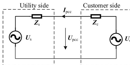
FIGURE 1. Thevenin equivalent circuit diagram.
