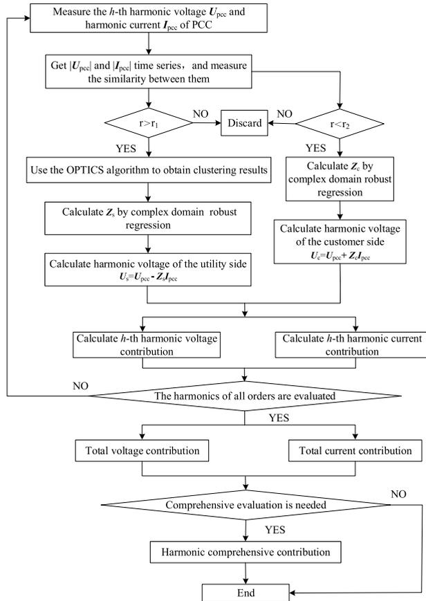
FIGURE 5. The process of harmonic contribution evaluation.
