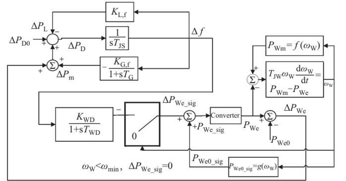
Fig. 7. Block diagram of droop control with time delay of the wind turbine generator.
