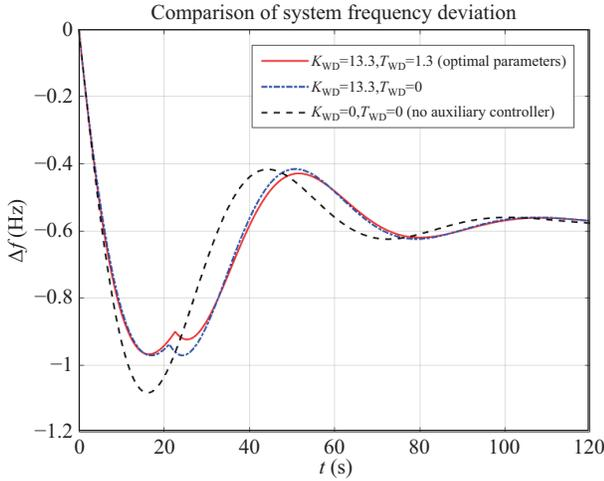
Fig. 9. The comparisons between SFRs with the auxiliary controller of optimal parameters and other parameters, and without controller.
