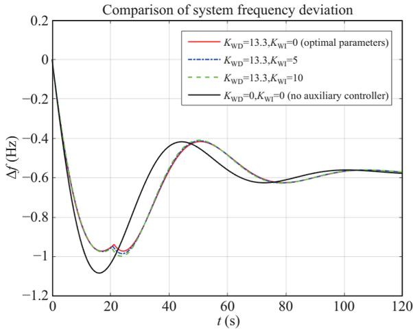
Fig. 6. The comparisons between SFRs with different parameters of controllers.
