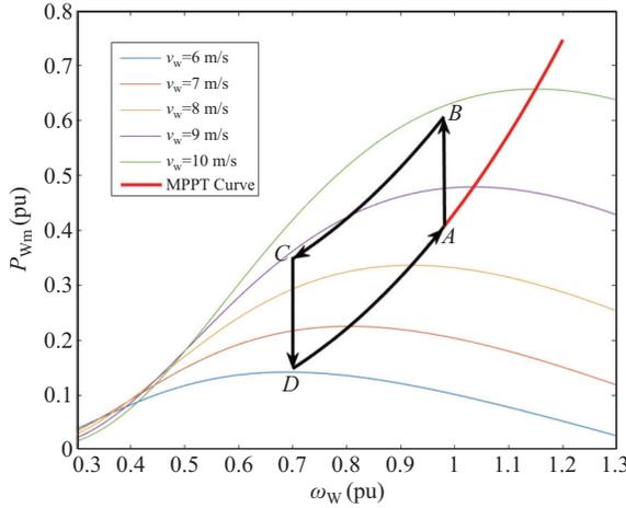
Fig. 2. Illustration of the entire process of participation of a wind turbine generator in power system frequency modulation when operating in MPPT mode.
