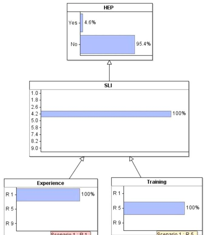
Fig. 2. BN-SLIM with deterministic PSF rates, representing the conventional SLIM.
