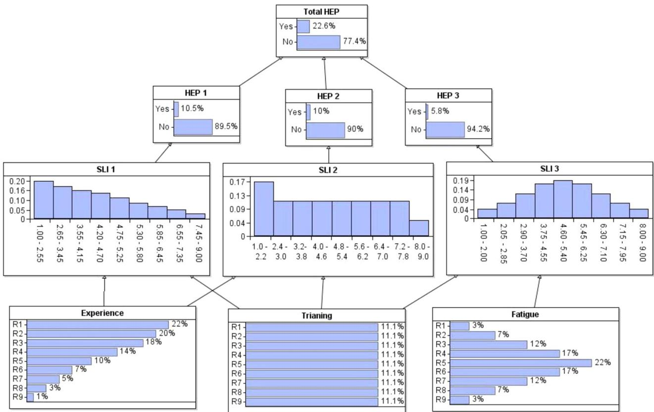
Fig. 3. BN-SLIM for the calculation of individual HEPs and the Total HEP.
