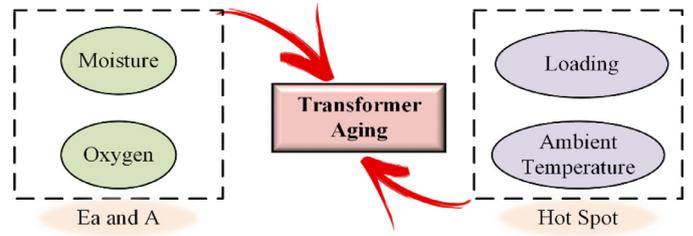
Fig. 1. The main players in the ageing procedure of oil-immersed transformers.
