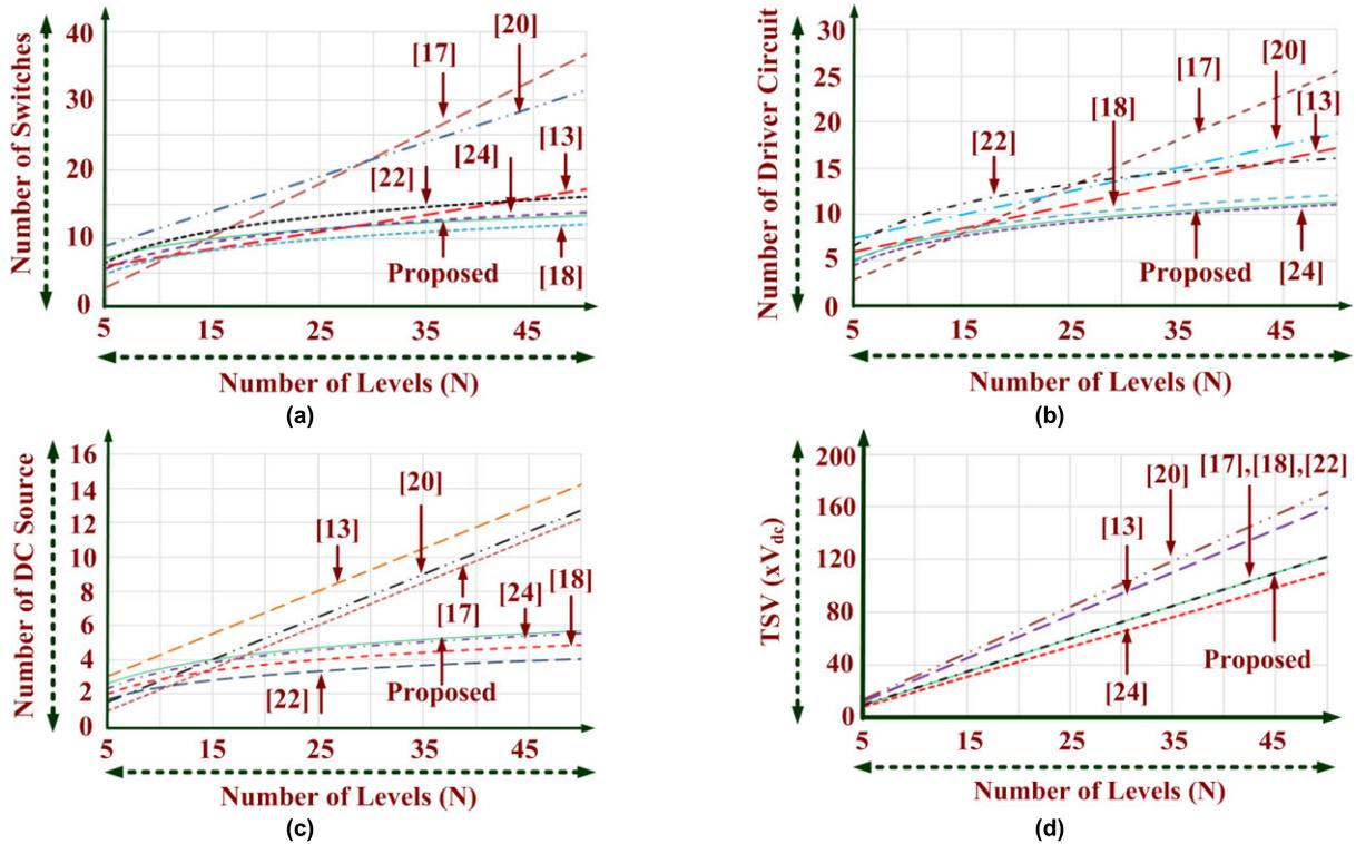
**FIGURE 6.** Comparison of asymmetrical configurations (a) number of levels, (b) number of driver circuits required, (c) number of dc voltage sources, and (d) TSV with respect of number of levels in asymmetrical mode of operation.
