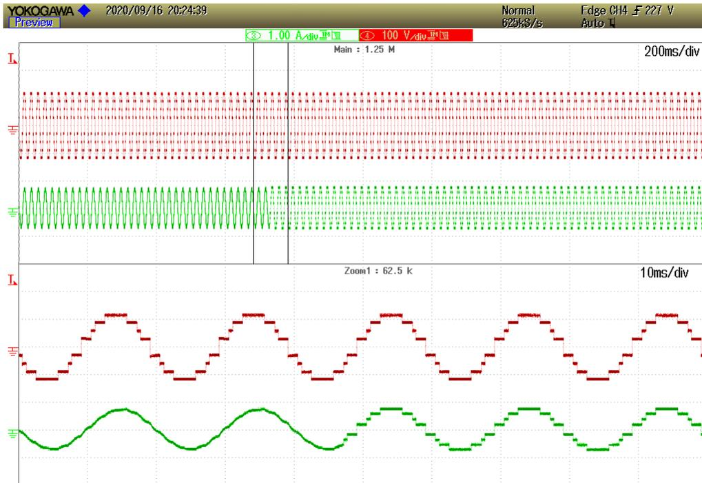
FIGURE 11. Output voltage and current waveform with change in load from RL to R load with symmetrical configuration.
