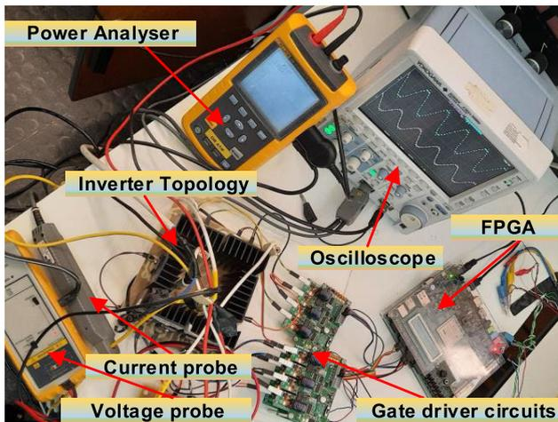
**FIGURE 7.** Hardware setup of the proposed MLI.
