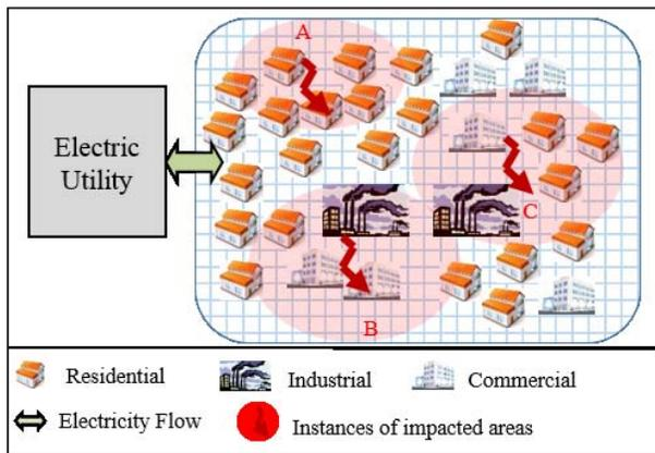
Fig. 2. Main entities of the distribution system model for reliability evaluation, and instances of impacted areas A, B, and C by different contingencies.
