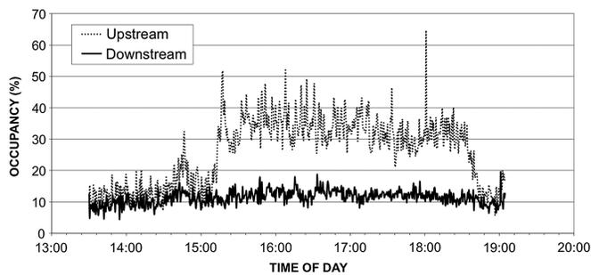
Fig. 3. Detector occupancy, SR 57 SB at Chapman Avenue, Fullerton.
