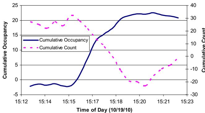
Fig. 4. Upstream detector cumulative curves.
