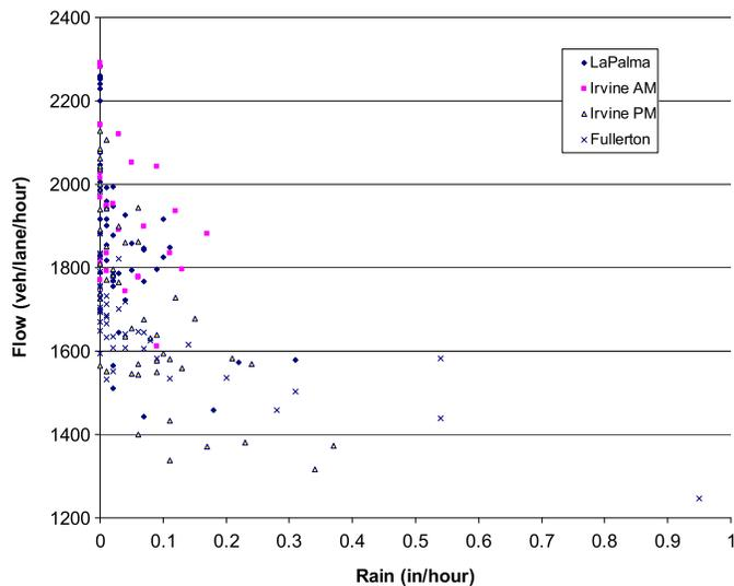
**Fig. 9.** Raw values of discharge flow for the four sites.
