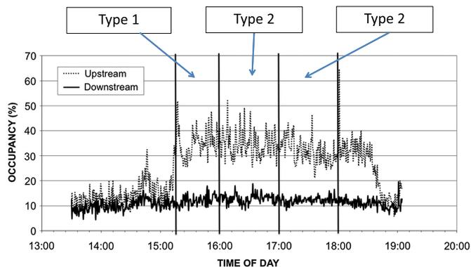
**Fig. 10.** Division of periods into two types, Fullerton bottleneck.
