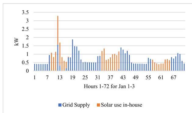
FIGURE 6. Grid and in-house solar usage for the household: Base Case.
