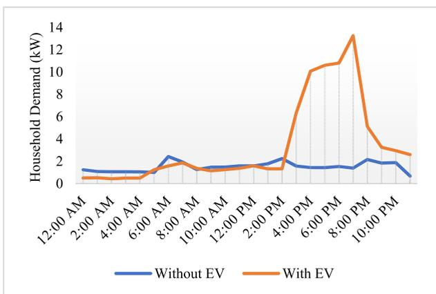
**FIGURE 2.** Smart meter data for a household without EV (2018) and with EV (2019) for July 3 (a weekday in both years).
