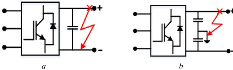
Fig. 2. DC microgrid fault (a) PP fault (b) PG fault.
