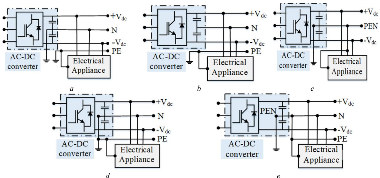
Fig. 4. Grounding system of DC microgrid (a) TT, (b) IT, (c) TN-C, (d) TN-S, (e) TN-C-S.
