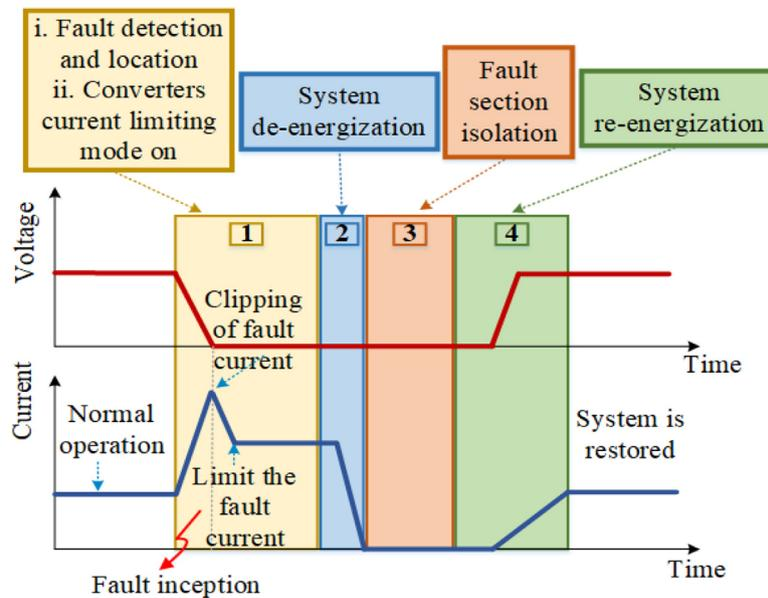
Fig. 6. Converter control action for fault mitigation [118].
