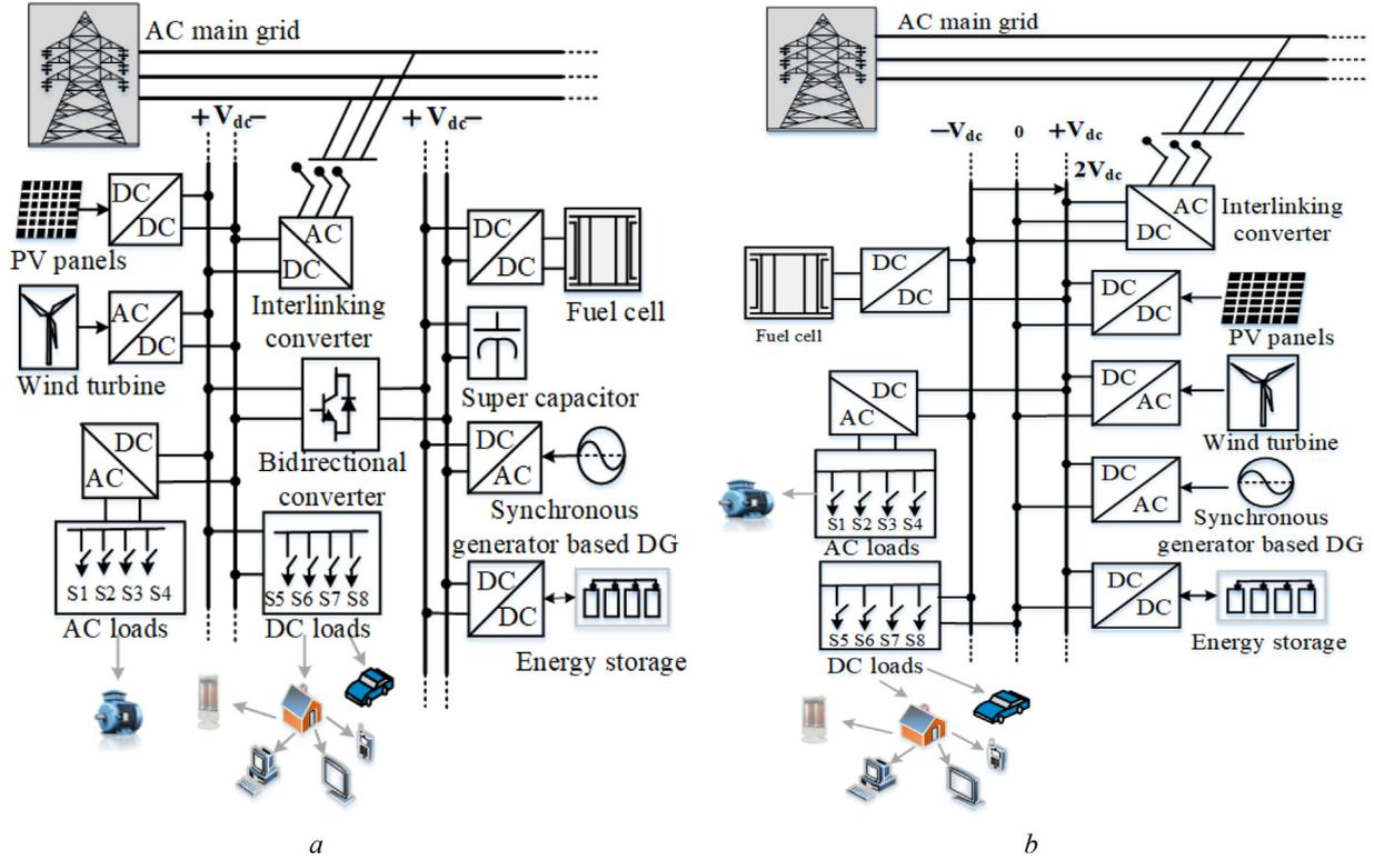
Fig. 1. DC microgrid polarity (a) Unipolar, (b) Bipolar.
