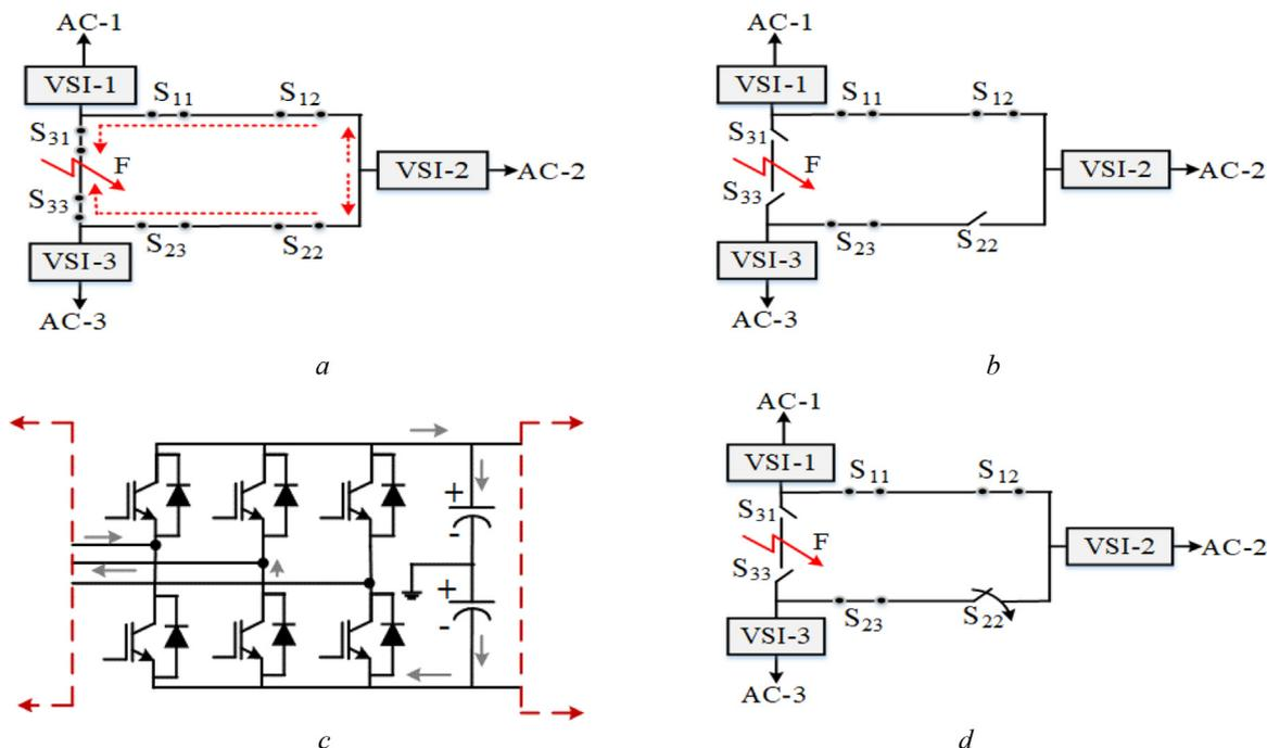
Fig. 7. Illustration of handshaking method [121], (a) Identification of the faulted line, (b) Opening of the faulted line, (c) Recharging of DC capacitors, (d) Reclosing of fast dc switch..
