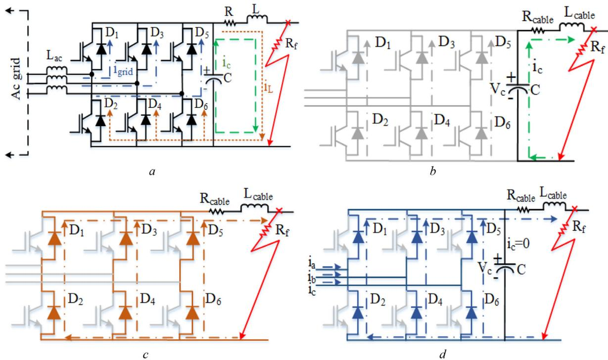
Fig. 3. DC fault current (a) DC cable fault in VSC, (b) stage-1:Capacitor discharge (c) stage-2:Diode freewheeling, (d) stage-3: AC grid feeding the fault.
