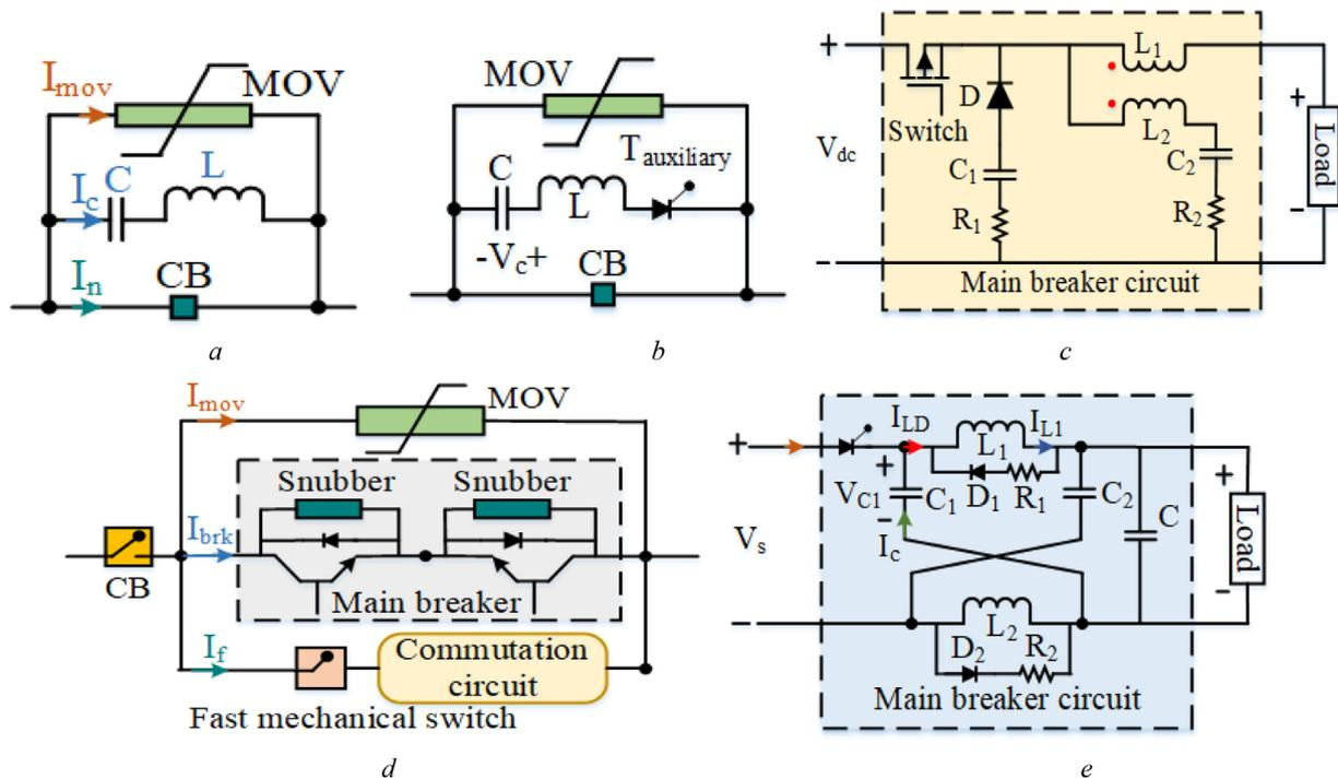
Fig. 8. DCCBs [18,19,35,74,162]. (a) MCB with passive commutation, (b) MCB with active commutation (c) SSCB, (d) HCB, (e) ZSCB.
