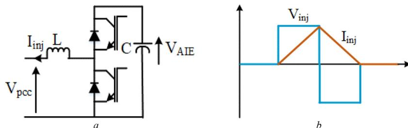
Fig. 5. Active impedance estimation technique [90] (a) Signal injector circuit, (b) Injected signal to the dc bus.
