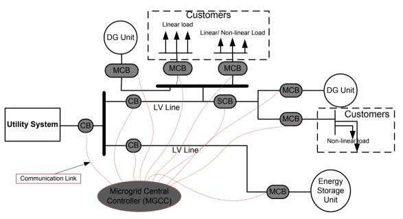
Fig. 2. Centralized protection system in AC microgrid system.
