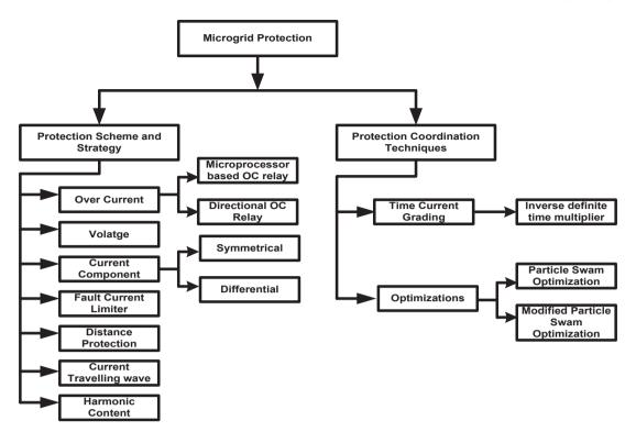
Fig.1. Protection schemes for microgrid operation.
