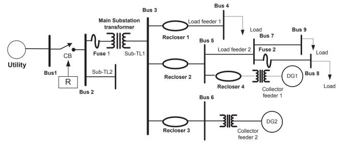
Fig. 8. the conventional time coordination between a CB, a recloser and lateral fuse for the distribution network comprising DGs.
