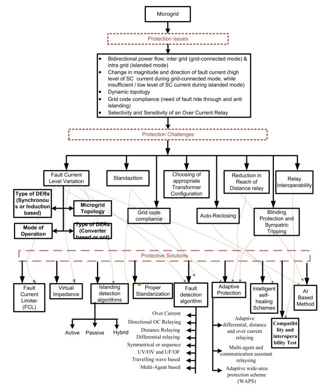
Fig. 6. Microgrid Protection issues, challenges and protective solutions.
