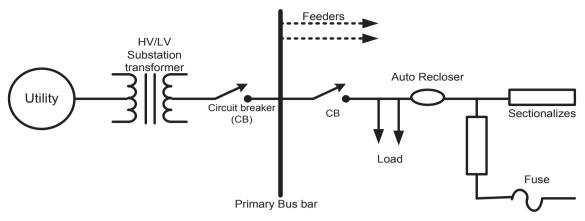
Fig. 7. Typical protection set-up for a simple radial feeder.
