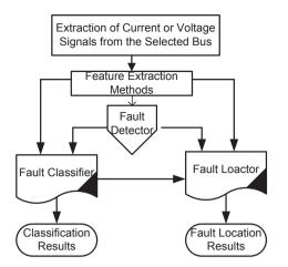
Fig. 9. Typical flowchart of fault detection, classification and location [184].
