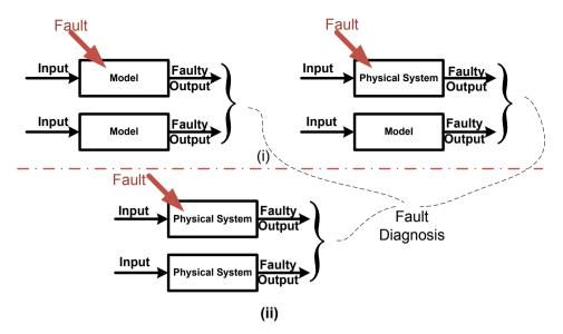
Fig. 3. Fault diagnosis approaches (i) Model Based methods (ii) Data-driven based methods.
