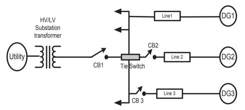
Fig. 5. A typical DG connections to a Distribution Network.
