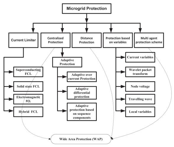
Fig. 4. Classification of microgrid protection schemes.
