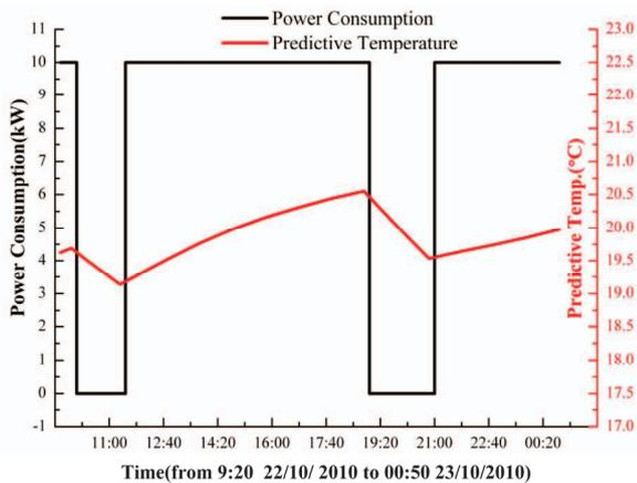
Fig. 7. Predictive indoor temperature in the next 15 hours
