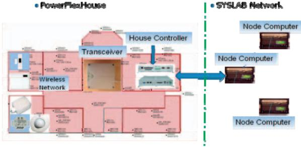
Fig. 3. Communication between PowerFlexHouse and SYSLAB
