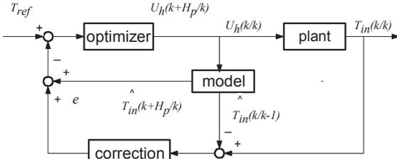
Fig. 5. Block diagram of PowerFlexHouse's MPC
