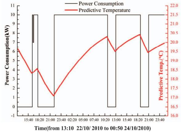
Fig. 9. Predictive indoor temperature in the next 35 hours
