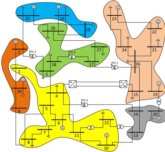
Fig. 5: Network clustering by ARMAX identification
