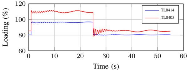
Fig. 7: Loading of transmission lines without power flow control
