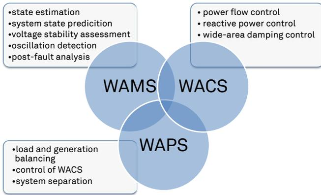
Fig. 1: Applications for wide-area monitoring, wide-area protection and wide-area control
