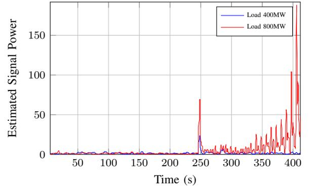
Fig. 6: ESPRIT based stability estimation at node 6
