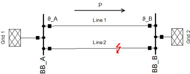
Fig. 9: A short circuit on an exemplary double line interconnector between Grid 1 and Grid 2.
