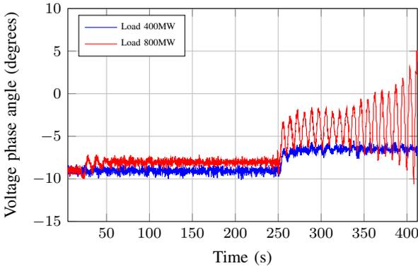
Fig. 2: Voltage phase angle at node 6 over time for different load situations in case of a line outage
