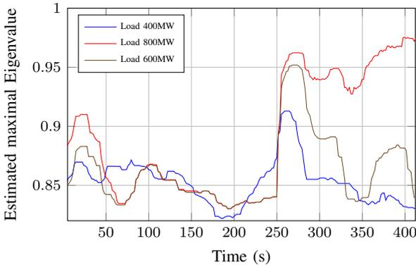
Fig. 3: ARMAX based stability estimation at node 6
