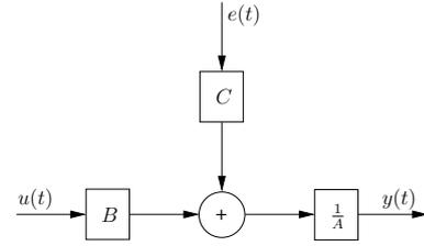
Fig. 4: Signal flow for ARMAX model
