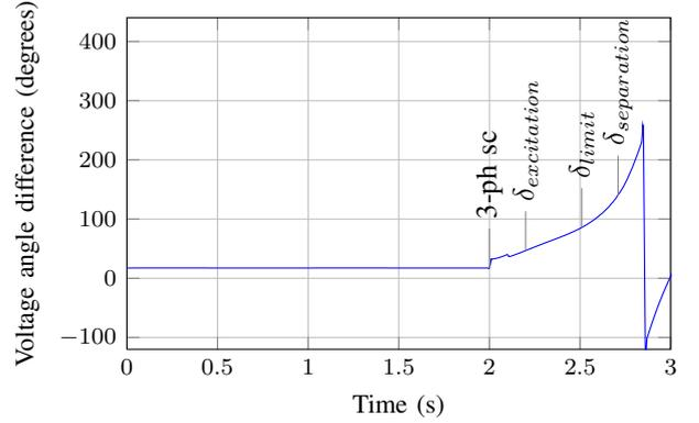
Fig. 10: Voltage angle difference between BB-A and BB-B
