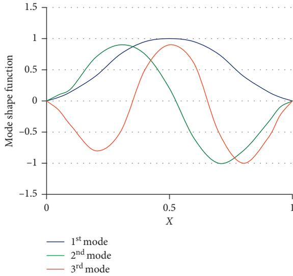
FIGURE 7: First three mode shapes for a clamped-clamped beam with  $K_0 = 1$  and  $\bar{P} = 1$ .
