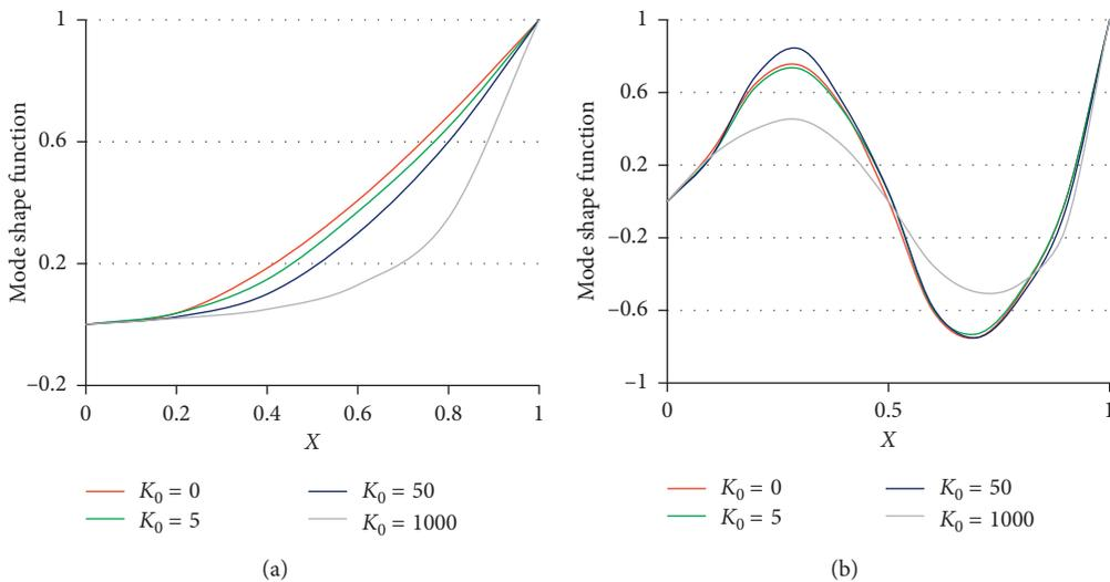
FIGURE 4: (a) First and (b) third mode shapes for various stiffness parameters with  $\bar{P} = 0$ .
