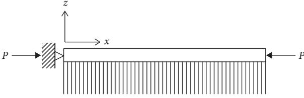
FIGURE 1: Beam under axial loading while resting on an elastic foundation.
