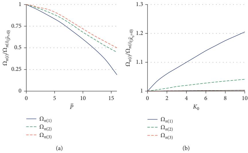
FIGURE 3: Variation of frequency modes with axial force and foundation stiffness.
