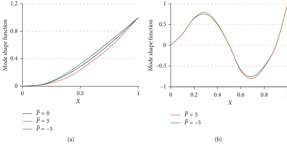
FIGURE 5: Effect of axial load on mode shapes with  $K_0 = 1$ . (a) 1<sup>st</sup> mode. (b) 3<sup>rd</sup> mode.
