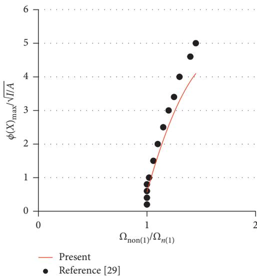
FIGURE 8: Comparison of backbone curves for the 1<sup>st</sup> mode of the clamped-clamped beam.
