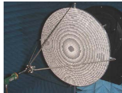
Fig. 12 Metal-only reflectarray antenna made of rectangular grooves for operating at 75GHz. (© 2011 IEEE. Reprinted, with permission, from [49]).
