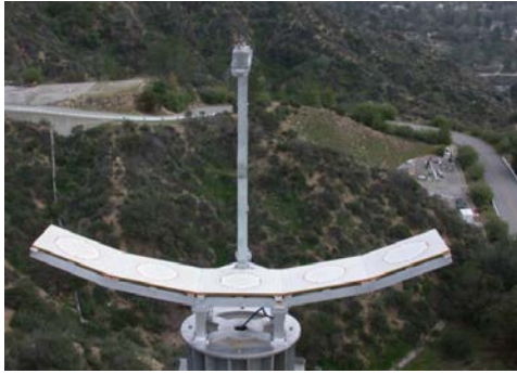
Fig. 16. Photo of the piece-wise flat reflectarray for WSOA in Ku-band (Courtesy of JPL, from [2] © 2008 John Wiley, Fig. 7.58)
