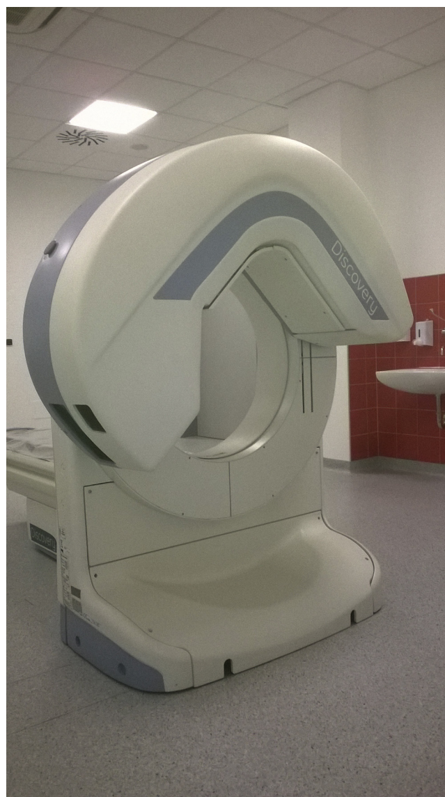
Fig. 2 – CZT camera with 90° arch of detectors (Discovery 530c, GE Healthcare).
