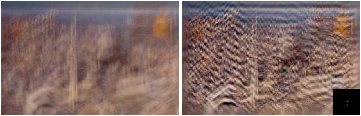
Figure 10: Failure case of the method on an image from Xu et al. [29]. Note that the described method was not able to correctly estimate the blur kernel since it is too large compared to the contrasted structures of the image.
