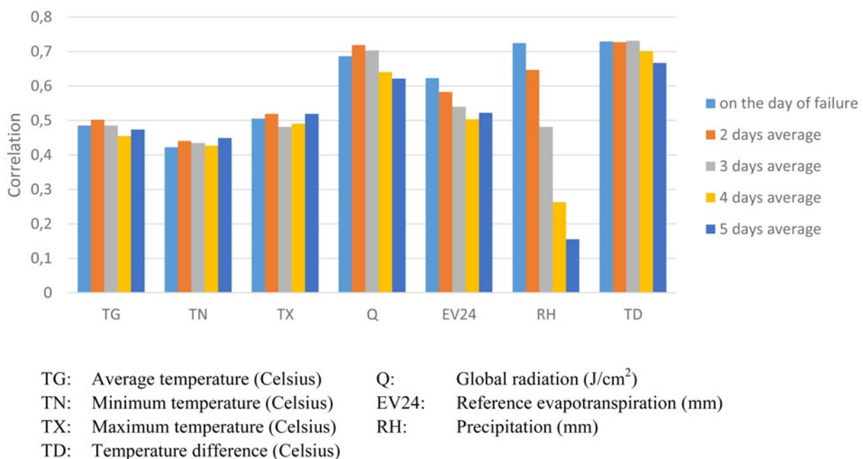
**Fig. 4** Correlation between failure rate of cable joints and weather conditions
