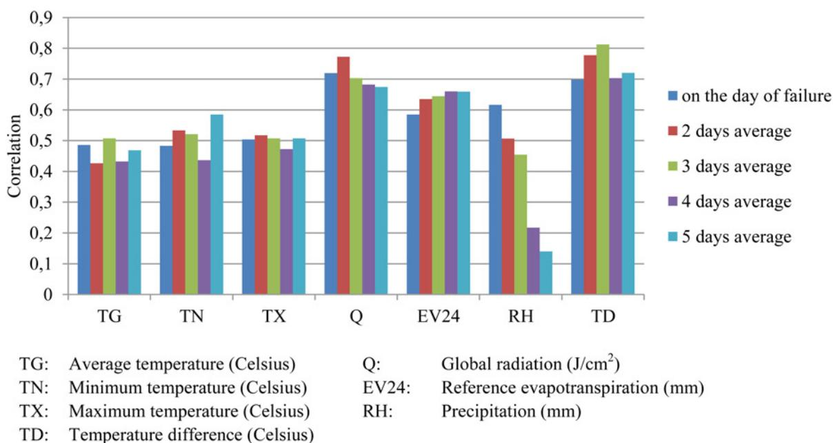
Fig. 3 Correlation between failure rate and weather conditions in Amsterdam area
