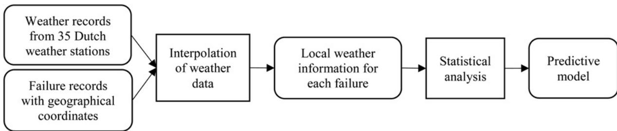
Fig. 1 Approach of investigating influence of weather conditions on failure rates
