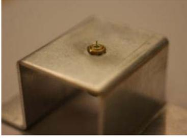
Fig. 2. *D*-dot sensor mounted on a grounded plane.
