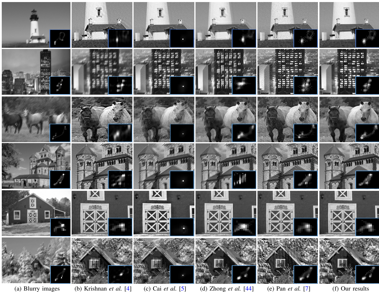
Fig. 8. Deblurring results on six image regions from the dataset by Sun et al. [17]. Note that the kernels estimated by the proposed algorithm are close to the ground truth data while the state-of-the-art methods tend to introduce noise in the estimated kernels. Although the kernels are estimated well by [7], the final deblurred images contain more noise than other methods. (images best viewed on a high-resolution display).
