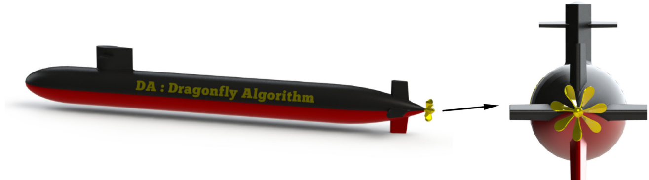
Fig. 19 A 7-blade propeller with 2 m diameter for submarines
