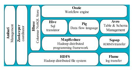
Figure 7. Common tools used in a Hadoop cluster.
