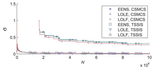
Fig. 4. Relationships between  $\sigma$  and the number of simulation runs under the CSMCS method and the TSSIS method respectively applied to IEEE-RTS79 with logarithmic ordinate axis. The TSSIS method is conducted with the denotation (b) for  $S_{II}(\Gamma)$ .
