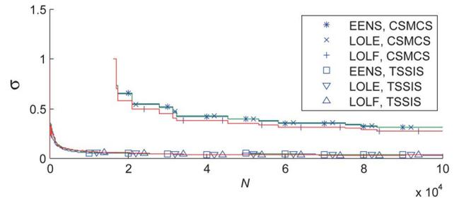
Fig. 3. Relationships between  $\sigma$  and the number of simulation runs under the CSMCS method and the TSSIS method respectively applied to IEEE-RTS79 with logarithmic ordinate axis. The TSSIS method is conducted with the denotation (a) for  $S_{II}(\Gamma)$ .
