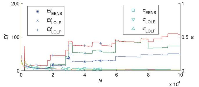
Fig. 9.  $Ef$  and  $\sigma$  of indices. The TSSIS method is conducted with denotation (c) for  $S_{II}(\Gamma)$  and load levels are independently Gaussian distributed.
