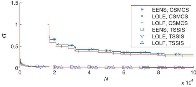
Fig. 5. Relationships between  $\sigma$  and the number of simulation runs under the CSMCS method and the TSSIS method respectively applied to IEEE-RTS79 with logarithmic ordinate axis. The TSSIS method is conducted with denotation (c) for  $S_{II}(\Gamma)$ .
