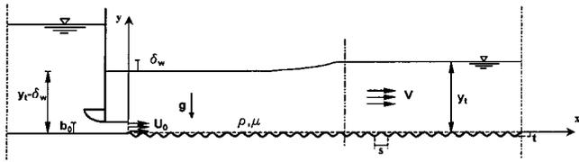
Fig. 1. Definition sketch for wall jets on corrugated beds
