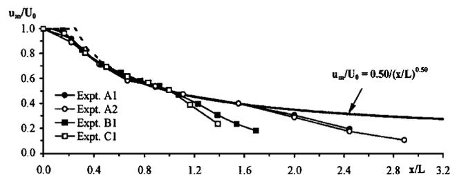
**Fig. 4.** Variation of the maximum velocity with distance
