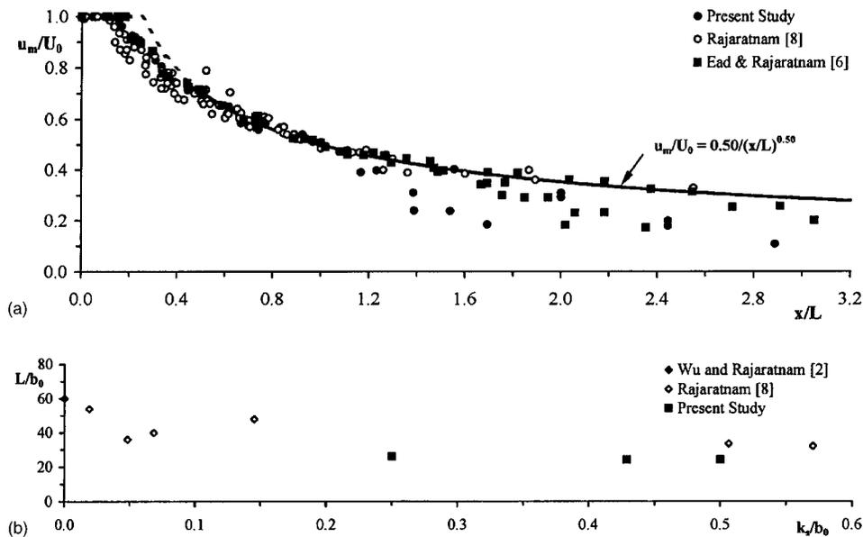
Fig. 6. (a) Variation of  $u_m/U_0$  with  $x/L$  and (b) variation of  $L/b_0$  with  $k_s/b_0$
