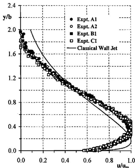
**Fig. 3.** Similarity profiles for the forward flow (all experiments)
