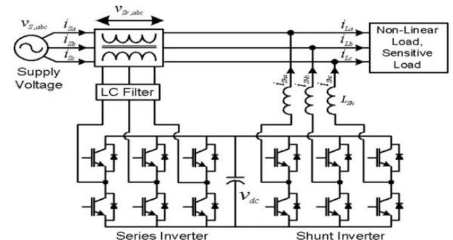
Fig. 8. UPQC of three phases three wires (3P3W)
