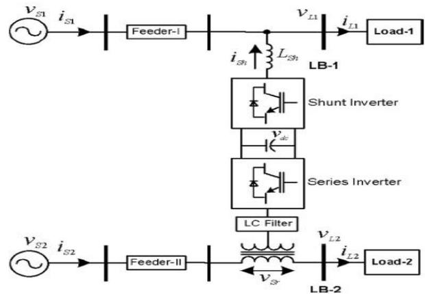
Fig. 10. system configuration UPQC-I
