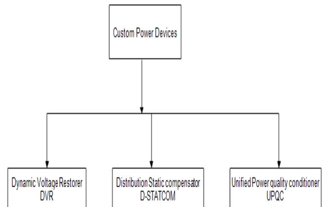
Fig. 1. Different types of custom power devices
