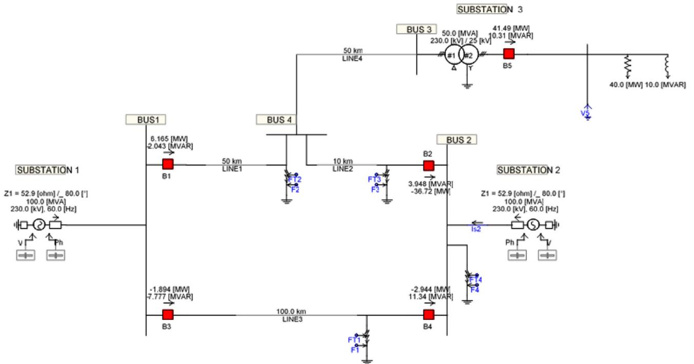
Figure 5 Single-line diagram of power system case study.
