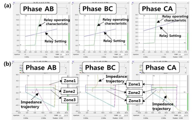
Fig. 6. In case of three-phase short circuit fault, the operation characteristic graph of relay when the fault occurred at F1.: (a) ~ (c) current differential relay, (d) ~ (f) distance relay.
