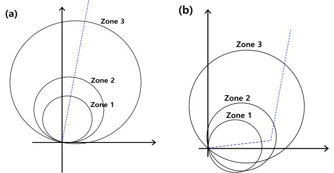
Fig. 1. (a) The case of Mho type characteristic: Application characteristic of only existing line impedance (b) The case of Mho type characteristic: Application characteristic of HTS cable impedance with existing line.
