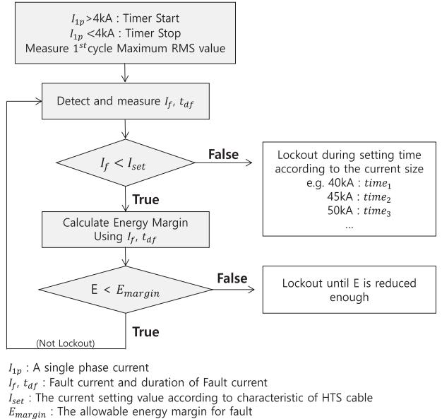
Fig. 3. The basic thermal protection algorithm of smart HTS cable.
