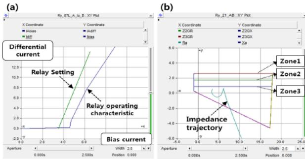
Fig. 5. In case of single line to ground fault, the operation characteristic graph of relay when the fault occurred at F1: (a) current differential relay (b) distance relay.
