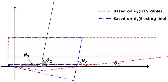
Fig. 2. The quadrilateral characteristic of relay based on line impedance angle: line impedance angle of both HTS cable and existing line.
