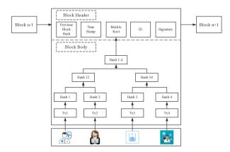
FIGURE 3. Block of blockchain-based EHRs.
