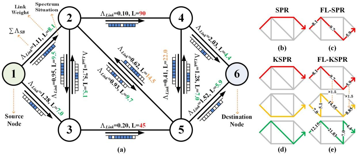
Fig. 3. Example of different routing schemes: (a) network topology and spectrum situation, (b) SPR scheme, (c) FL-SPR scheme, (d) KSPR scheme, and (e) FL-KSPR scheme ( $k = 3$ ).
