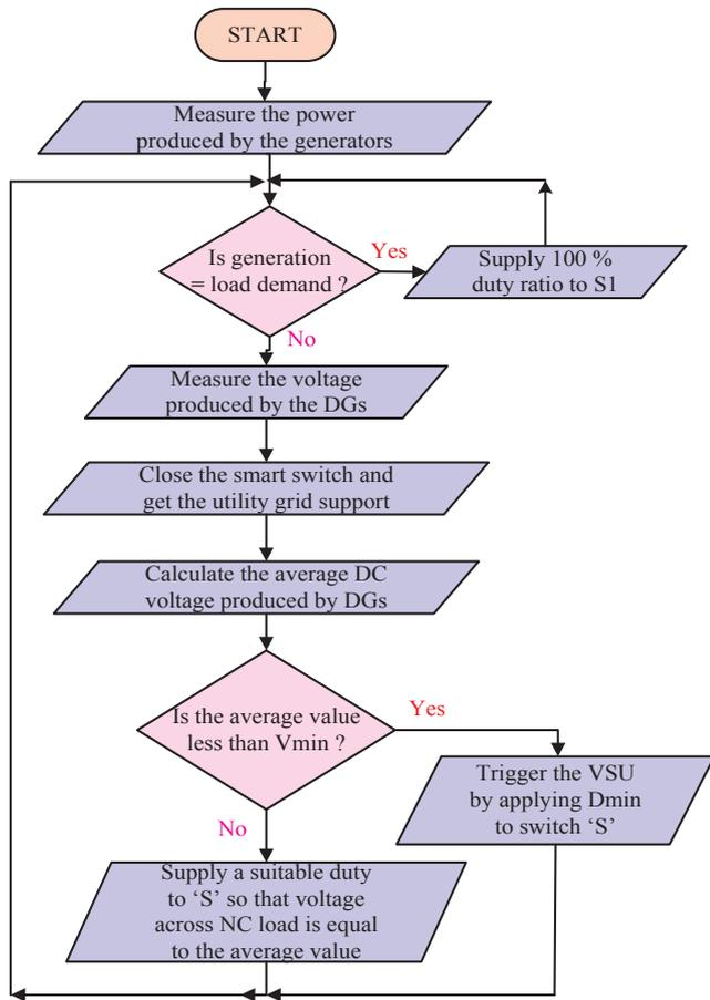
Fig. 4. Flow chart of the rule based energy management algorithm.
