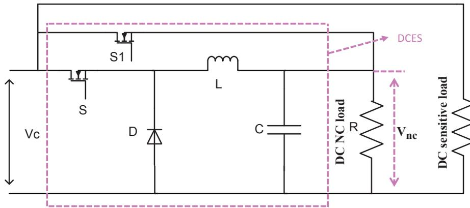
Fig. 2. Connection diagram of the DCES or the virtual storage unit [28].
