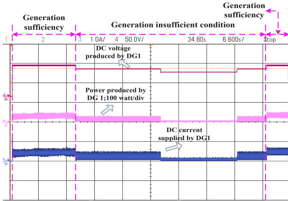
Fig. 6. Output DC parameters of the DG1.
