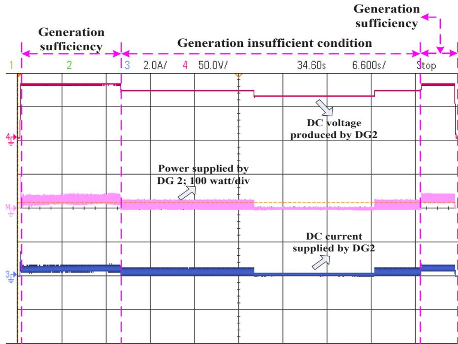
Fig. 7. Output DC parameters of the DG2.
