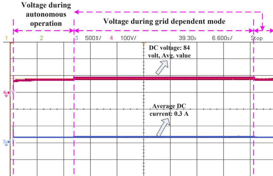
Fig. 9. Voltage and current supplied to the DC sensitive load.
