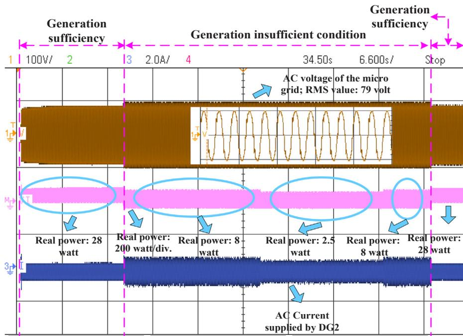
Fig. 12. AC power supplied by the DG2.
