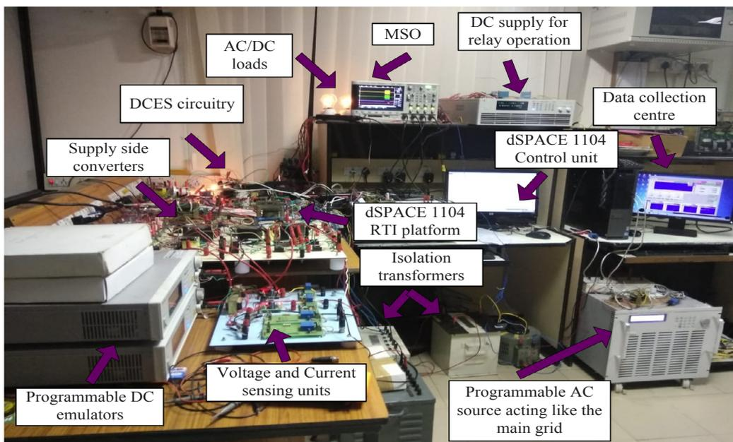
Fig. 5. Laboratory scale hybrid micro grid developed for the study.
