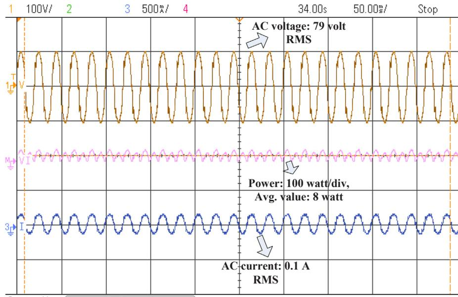
Fig. 8. AC sensitive load parameters.
