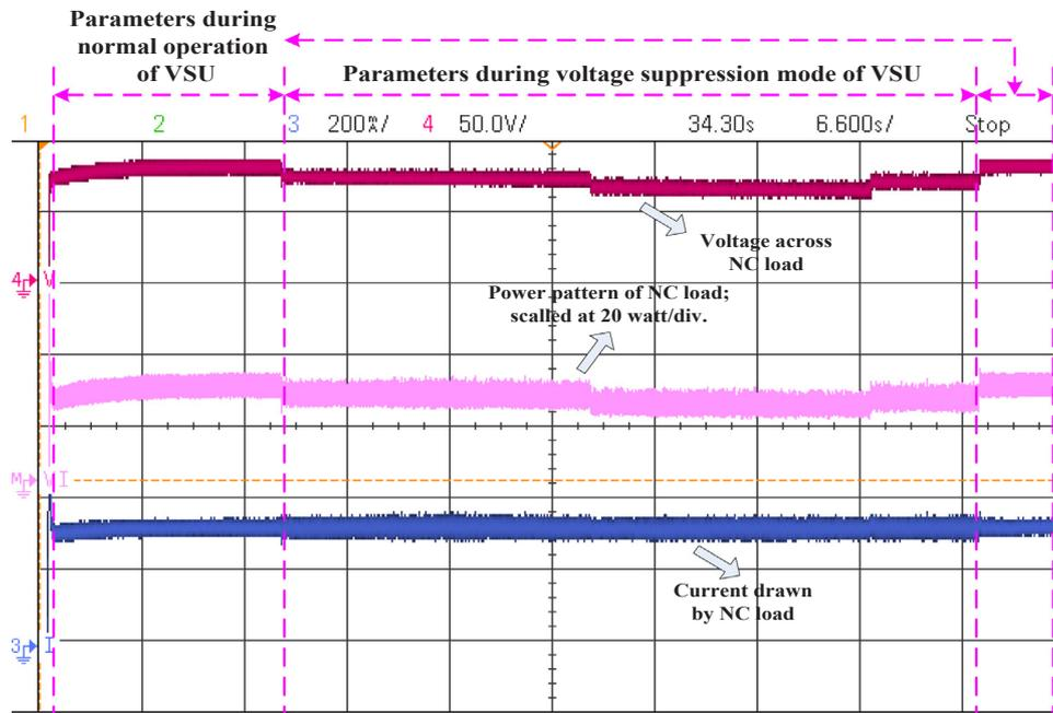
Fig. 10. Parameters of the NC load.
