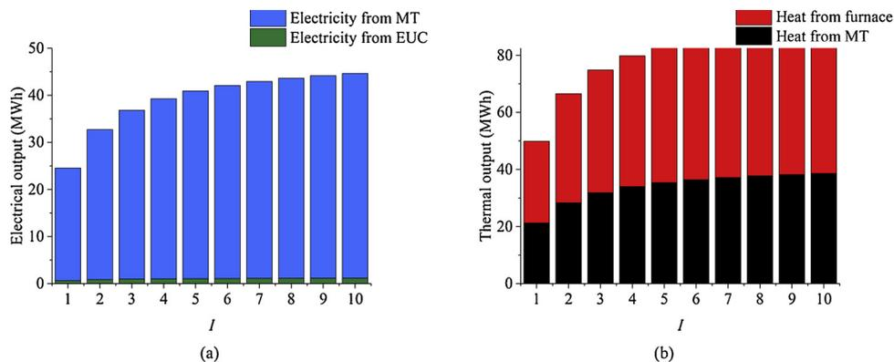
Fig. 8. Composition of the total energy outputs of the S.E. hubs when the number of S.E. hubs changes ( $K$  is fixed at 4): (a) electrical output; (b) thermal output.
