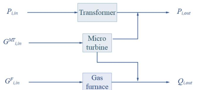
Fig. 2. Schematic diagram of the smart energy hub in the IES.
