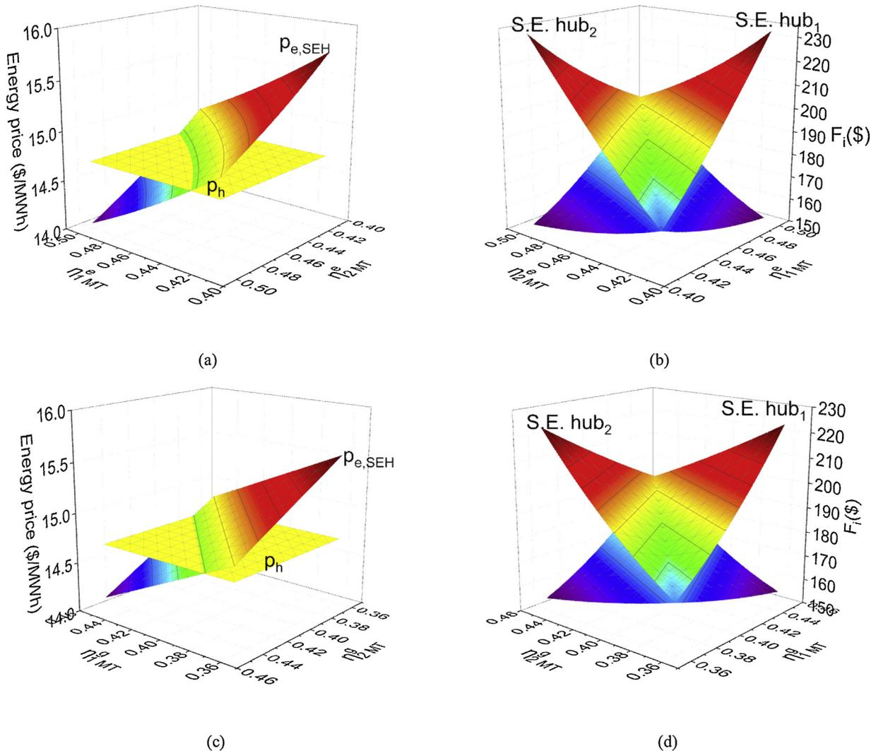
Fig. 10. Impact of the efficiencies of the micro turbines: (a) impacts of  $\eta_{i,MT}^e$  on the energy prices; (b) impacts of  $\eta_{i,MT}^e$  on the profits of S.E. hubs; (c) impacts of  $\eta_{i,MT}^g$  on the energy prices; (d) impacts of  $\eta_{i,MT}^g$  on the profits of the S.E. hubs.
