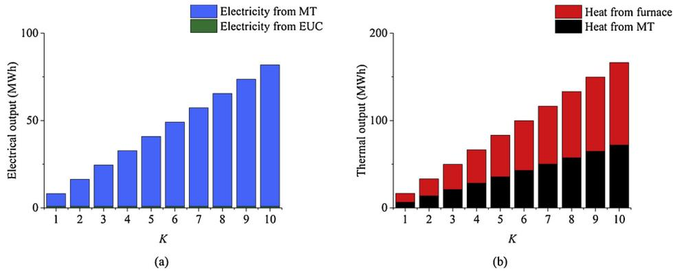
Fig. 9. Composition of total energy outputs of the S.E. hubs when the number of users increases ( $I$  is fixed at 2): (a) electrical output; (b) thermal output.
