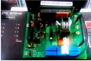
Fig. 5. Si-IGBT test platform (ITC57240).
