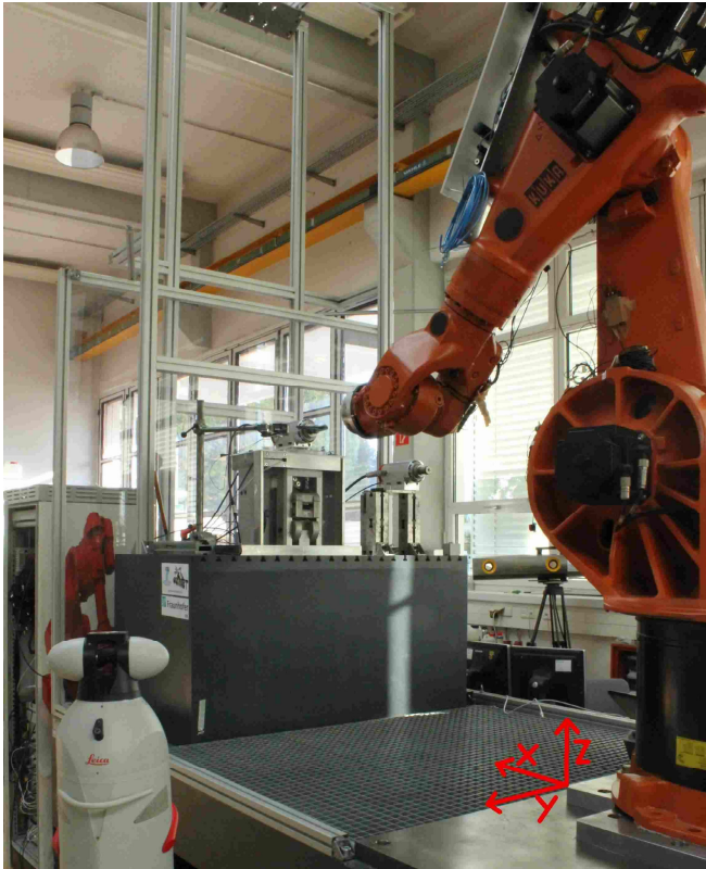
Fig. 6. Experimental setup with machine bed, KR125 robot, Chopper 3300 spindle, Keyence LK-G87 sensor and Lasertracker
