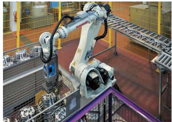
Fig. 4: separation of unsorted parts in a cage by a robot using a vision system (Fraunhofer IPA)
