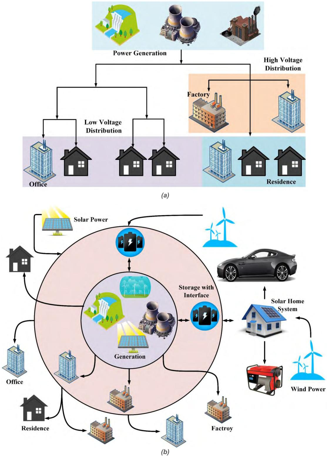
**FIGURE 1.** Utility grids: (a) conventional grid (b) smart grid. In the conventional system power flows from in one direction only; but for smart grid, there is no strict structure. Generation can occur at the consumer side too, such as the wind and the solar farms at the outer periphery of the topology. Power flow can also be bidirectional, demonstrated by the energy storages and the house in this illustration.
