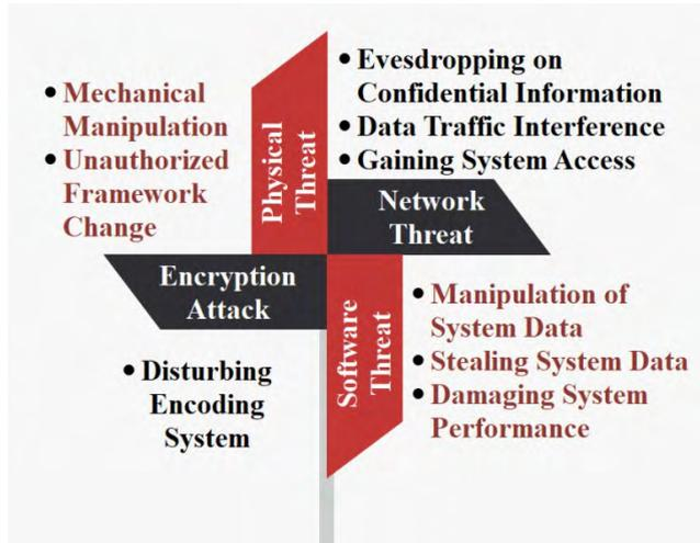
**FIGURE 10.** Security concerns of IoT integrated SG system. These can be categorized into four major types: physical threat, network threat, software threat, and encryption threat. The security concerns under each type are marked in corresponding color.
