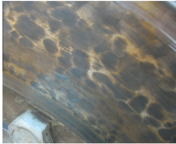
Fig. 1. Hotspots on the friction surface.
