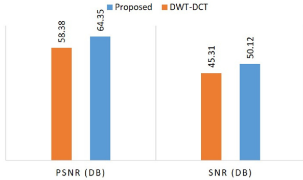
Fig. 8. PSNR (dB) and SNR (dB) using the proposed DWT-SVD based watermarking, which is compared with DWT-DCT based watermarking.
