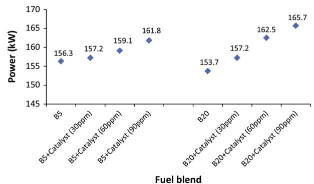
**Fig. 4.** Results of maximum power generated by different fuel blends (B5 and B20) containing CeO<sub>2</sub>-MWCNTs nanocatalyst at the speed of 1500 rpm and full load.
