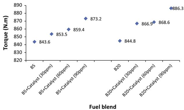
Fig. 5. Results of maximum torque by different fuel blends (B5 and B20) containing CeO<sub>2</sub>-MWCNTs nanocatalyst at the speed of 1500 rpm and full load.
