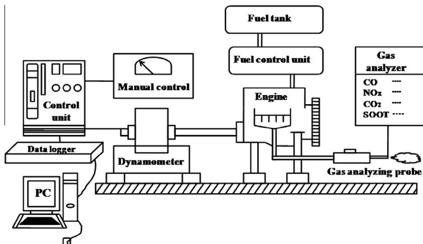
Fig. 1. Schematic figure of the diesel test engine setup.
