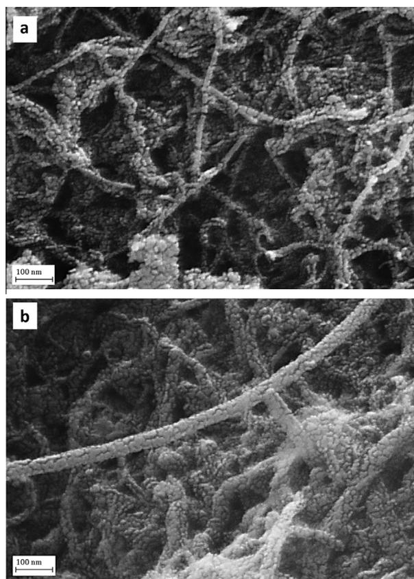
Fig. 3. Scanning electron microscopy (SEM) micrographs of the MWCNTs, (a) prior to hybridization/amidation processes and (b), the amidated  $\text{CeO}_2$ -MWCNTs.
