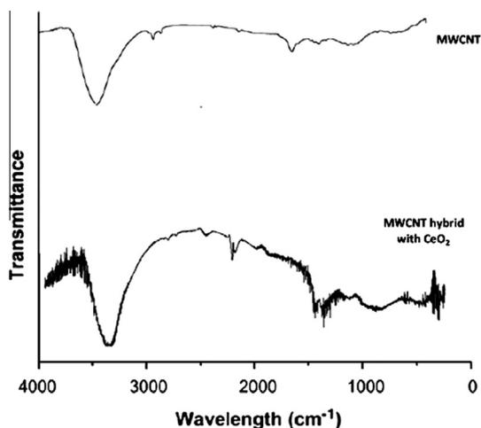
Fig. 2. The FTIR spectra of the MWCNTs and the amidated  $\text{CeO}_2$ -MWCNTs.
