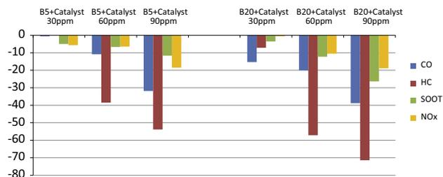
**Fig. 7.** Overall decrease in emissions (i.e., CO, HC, Soot and  $\text{NO}_x$ ) achieved by addition of the  $\text{CeO}_2$ -MWCNTs nanocatalyst at different concentrations (30, 60 and 90 ppm) compared to catalyst-free B5 and B20.
