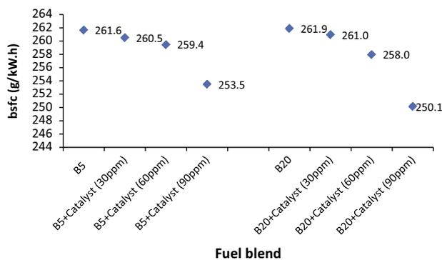
Fig. 6. Results of bsfc for different fuel blends (B5 and B20), and at different CeO<sub>2</sub>-MWCNTs nanocatalyst inclusion rate i.e., 30, 60 and 90 ppm at the speed of 1500 rpm and full load.
