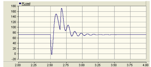
(b) active power of load with induction motor(kW)
