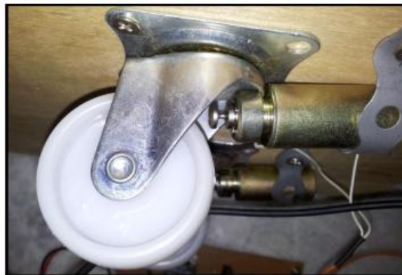
Figure 1: Simple locking mechanism proposed by N. Othman [1]
