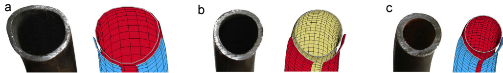
Fig. 7. Cross-section of tubes bent on a MDB-Die, \theta = 150^\circ , D = 25 mm. (a) d = 25 , t = 2 , (b) d = 20 , t = 2 , (c) d = 18 , t = 2.5 .
