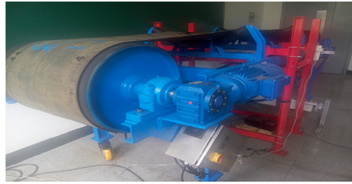
Fig. 11. Belt conveyor for test in laboratory.
