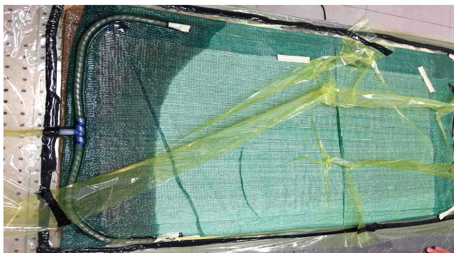
Figure 1. VARI processing adopted to manufacture SMA/GF/epoxy hybrid composite laminates.
