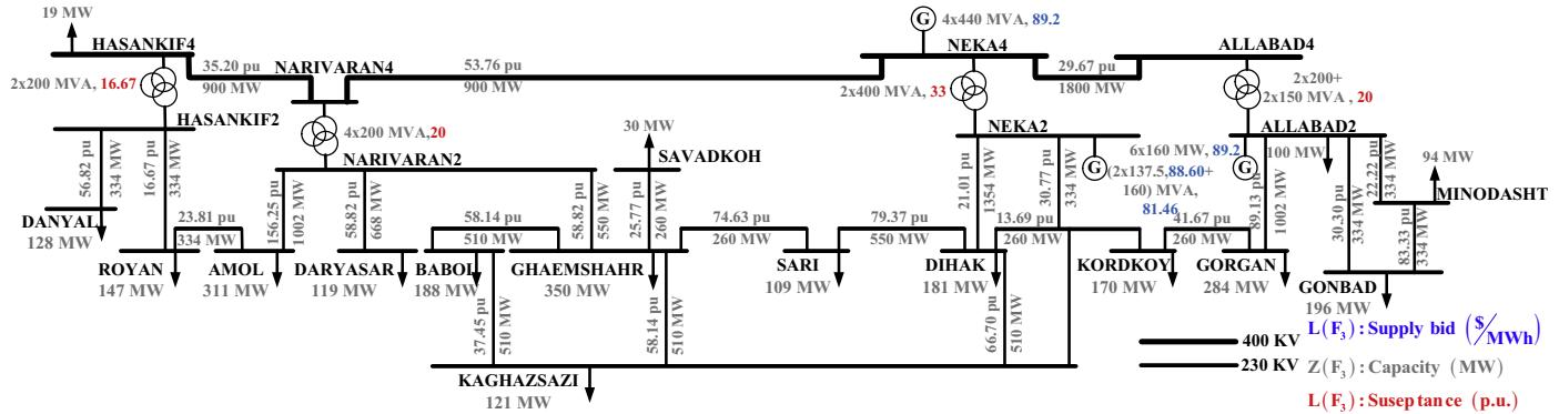
**Fig. 5.** Single-line diagram of MREC transmission network.**Table 3**
