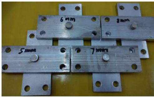
Fig. 6 Mechanical property samples after the EMR process
