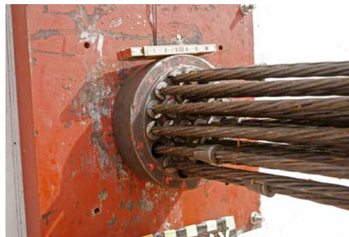
Wedge Unseating – Explosive Tests
